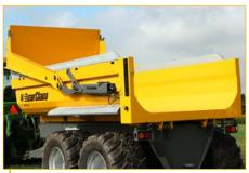
End gate flips into up position so stumps and branches don't get snagged when dumping.
