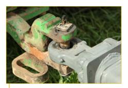
Swivelling ball hitch reduces wear on drawbar.
