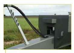
Hydraulic hoses enter welded frame at base of tongue to reduce snagging of hoses.
