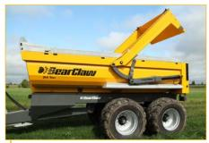
High clearance end gate for hauling stumps and tree branches.
